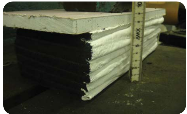
Flexi®-Coat @ 2.5mm WFT cured on to elastomeric substrate to perform dynamic tests.
